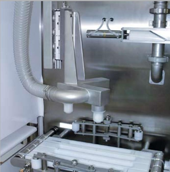
In cheese production the food-safe Franke Dynamic Aluminium Roller Guide provides the vertical movement of a grappler for wheels of cheese. In this application it is important that the roller guide is insensitive to whey and aggressive cleaning agents.
