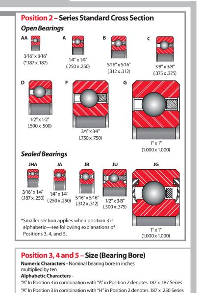
**Examples -** 040 = 4.0" Bore, 120 = 12.0" Bore, 400 = 40.0" Bore "10" following "AA" in Positions 2 &  $3 = .187 \times .187$  Series with 1.0" Bore
