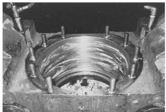
Fig.11 Chock bore before installing
