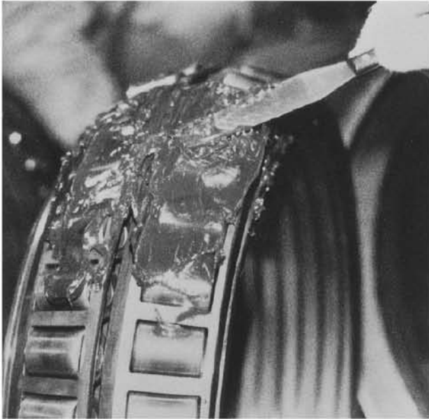
Fig.16 Fill the grease in cone assembly.
