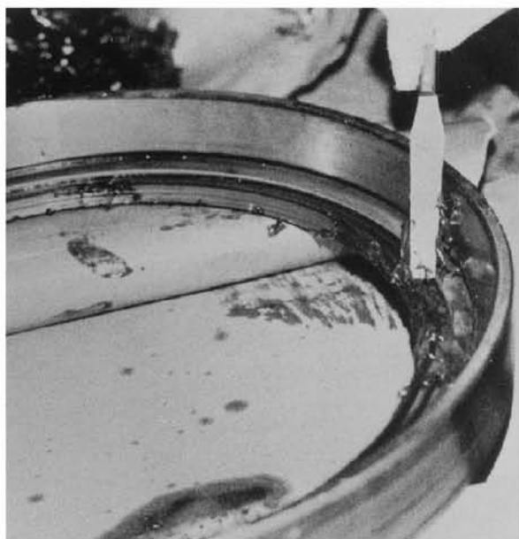
Fig.15 Coat the grease on cup raceway
