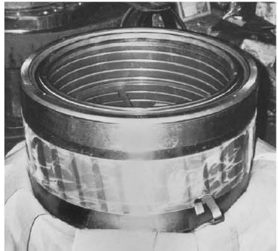
Fig.9 Packing off the bearing
