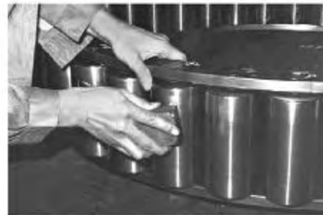
Photo. 3-5 Correction of roller rolling surface (Oil stone)
