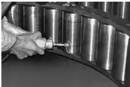
Photo. 3-4 Correction of roller rolling surface (Microgrinder)
