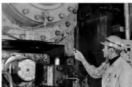
Photo. 3-1 Checking sound with soniferous bar
