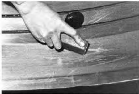
Photo. 3-2 Correction of outer ring raceway surface (Oil stone)
