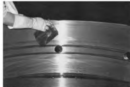
Photo. 3-3 Correction of outer ring raceway surface (Emery cloth)
