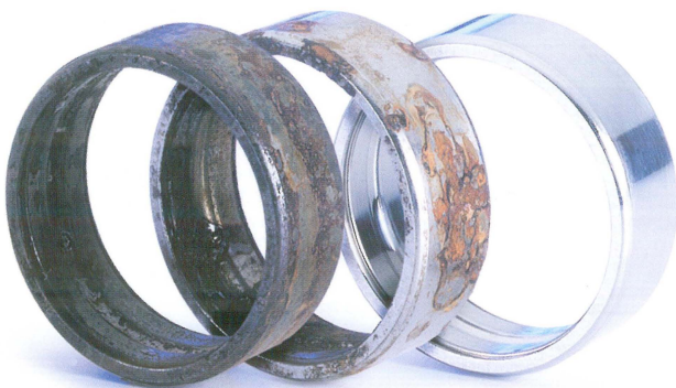
Figure 4: Comparison of corrosion rate 52100, X65Cr13 and SV30
