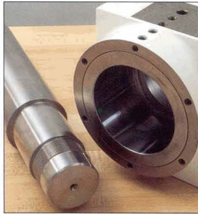
It is critical that shafts and housings be clean, burr-free and machined to exact tolerances.
