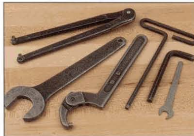
Use clean, burr-free tools that are not plated, painted or rusted.
