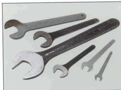
OPEN END WRENCHES Always use unplated tools.
