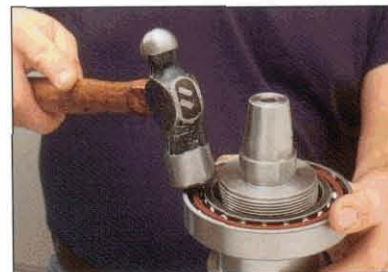
Don't use a hammer or screwdriver to install bearings. Never drop bearings.
