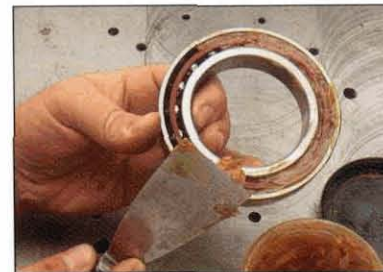
Don't over lubricate or mix different lubricant families.
