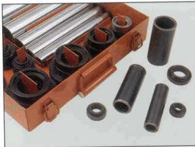
DRIFTS Facilitate ring installation.
