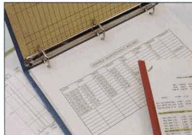
Keep maintenance logs and record bearing nomenclature from box.
