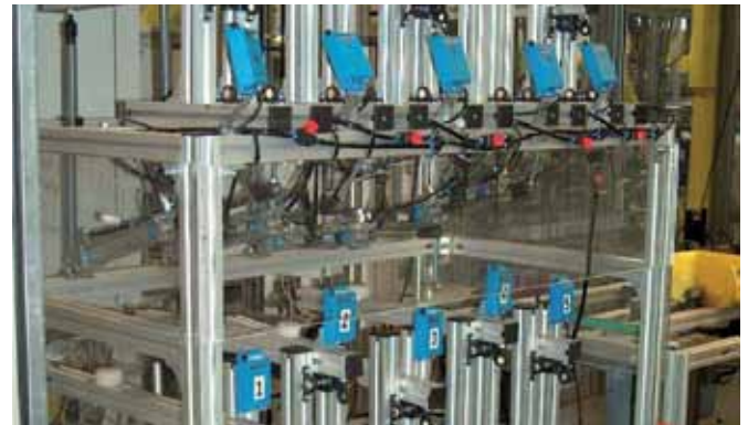
Oscillating wear test rig for testing the wear in oscillating movements at medium loads
