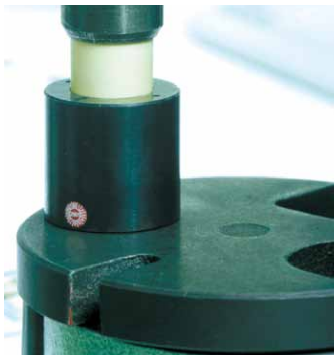
The bearing should be press fitted using a flat press.
