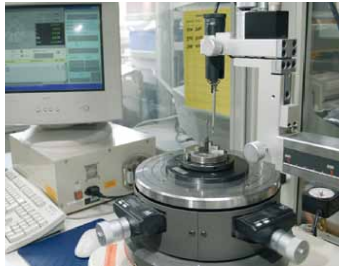
Measurement of the inner diameter of a pressfit plain bearings
