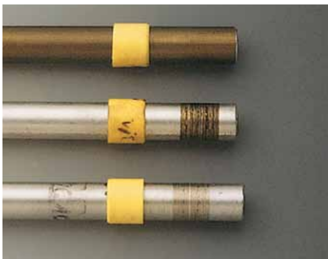
Wear experiments with aluminum shafts
