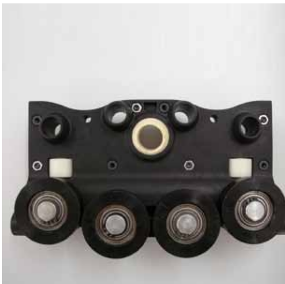
Carriage in a crane system
