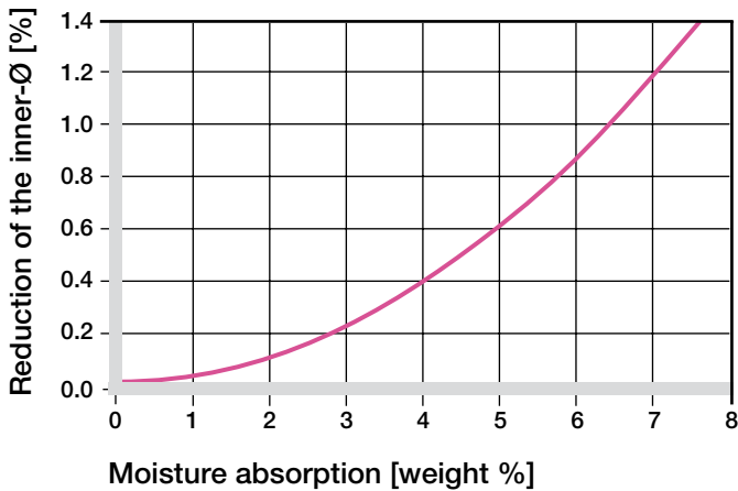
Graph 10: Effect of moisture absorption on plain bearings
