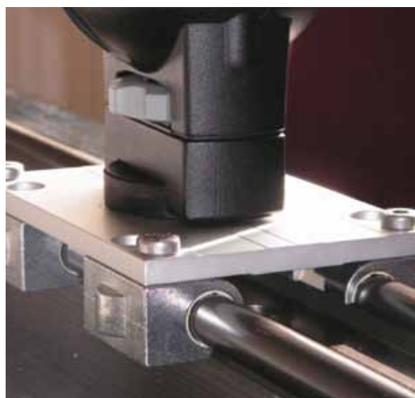
Adjustment of camera mounting slide
