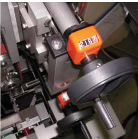
Size adjustment in bag forming, filling and sealing machine with DryLin® SET
