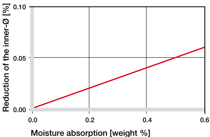
Graph 10: Effect of moisture absorption on plain bearings
