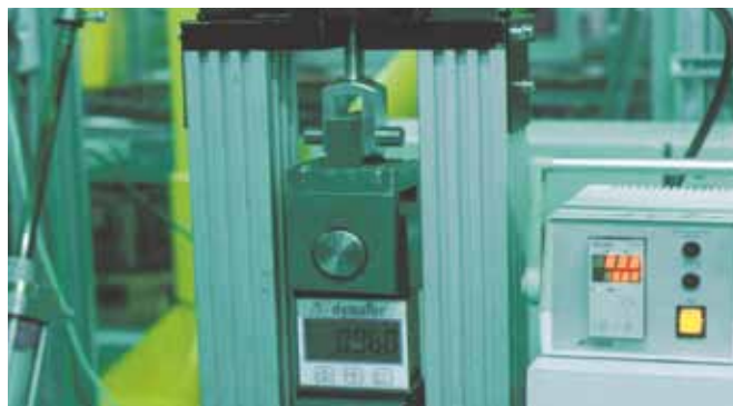
Test bench for loads up to 150 MPa and temperatures up to +250 °C
