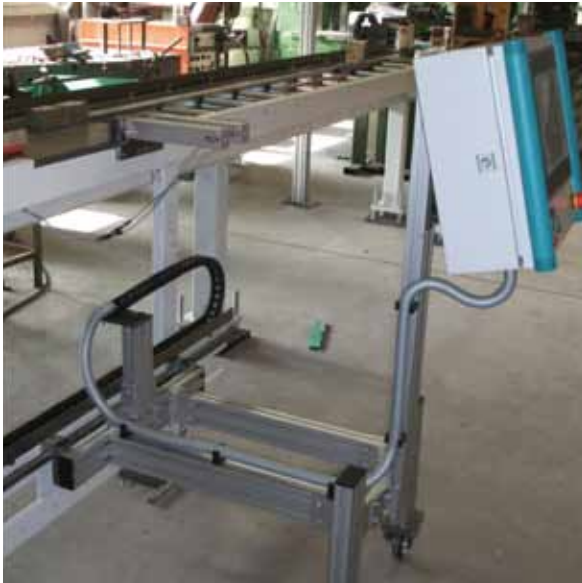
Adjustment of control panel unit
