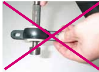
Inadequate test equipment; mandril gauge to short
