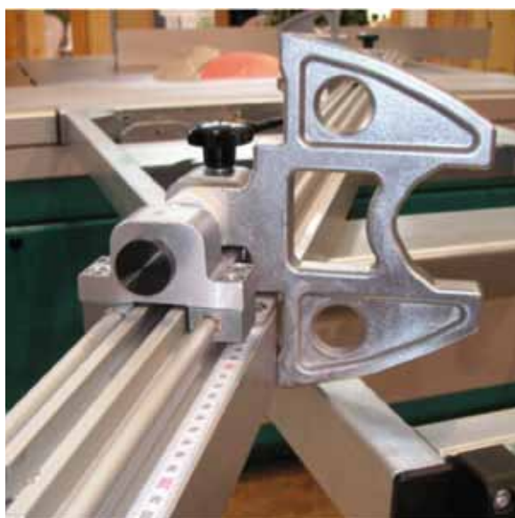
Stop dog system of a sliding table panel saw
