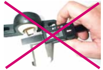
Wrong test equipment; caliper
