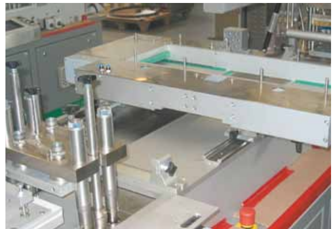
DryLin® W is accredited to Cleanroom-set points and in use in this blister machine.
