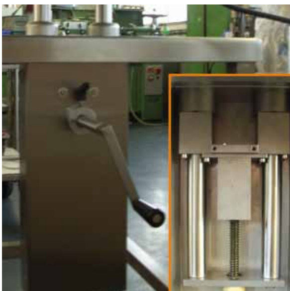
Can opener: drive for the height adjustmet
