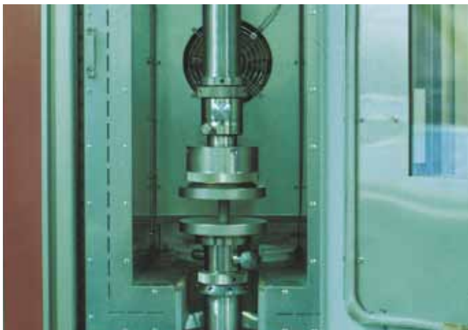
Material tests are possible up to +250 °C
