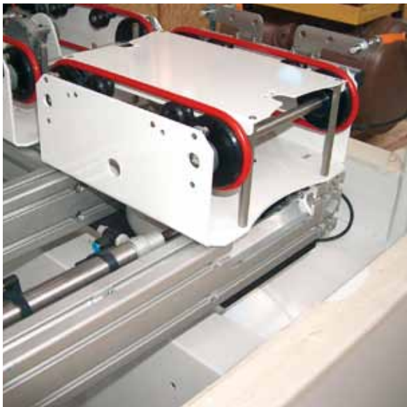
Handling and conveyance system for semiconductor transport/box.
