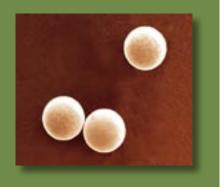
Bow<sup>®</sup> Electronics products are known for their consistently high performance in quality-critical electronic applications. One of the newest Bow Electronics innovations is high-precision copper spheres. Produced by a proprietary process which eliminates surface cracks and craters, the copper spheres are perfectly round to provide a narrower process window and improve reliability. They are an ideal replacement for traditional lead and tin alloys.
