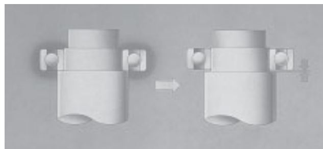
● Figure 9.3 Shaft Shoulder Gap After Cooling
