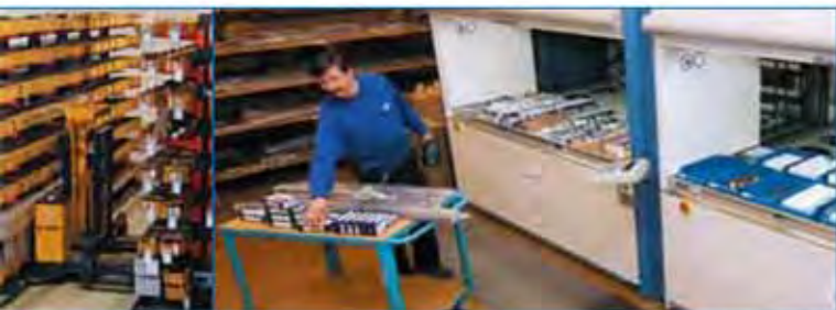
Shuttle systems combined with a bar code system allow fast access and fast cycle times in the Stuttgart warehouse.
