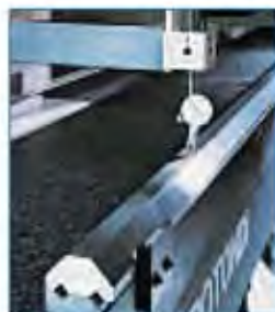
Straightness measurement using a GU series linear guide track
