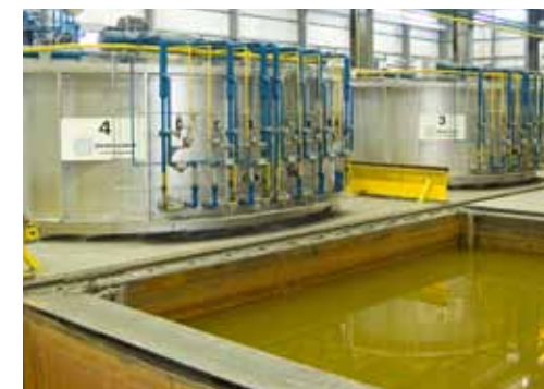
Eight heat treat furnaces and multiple quench tanks.
