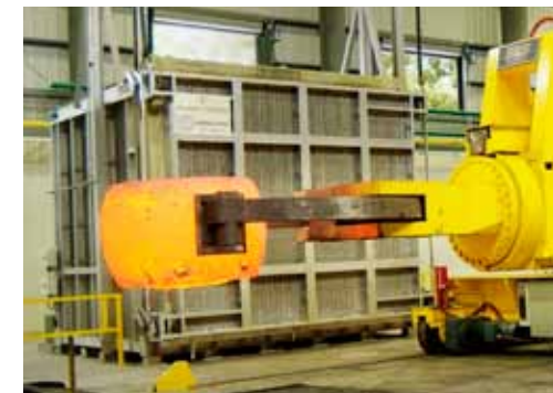
Manipulator transfers ring from furnace to mill.
