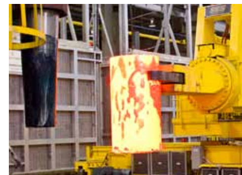
Manipulator transfers billet from furnace to press.
