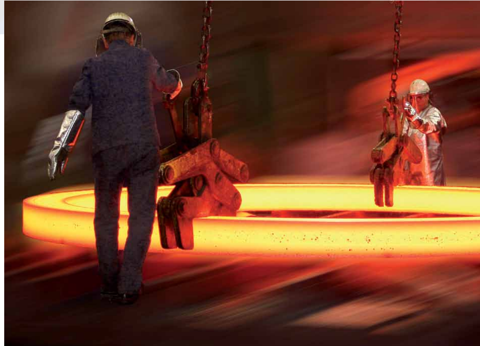
Manipulator transfers ring from furnace to mill.
