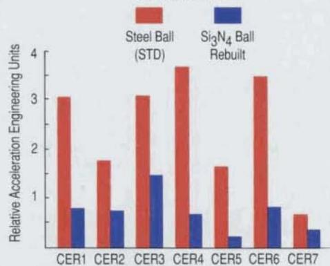
**FIG. 6:** Vibration tests comparing spindles with steel ball bearings and the same spindle retrofit with ceramic hybrids. Vibration levels averaged two to seven times lower with silicon nitride balls.
