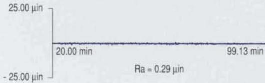
**FIG. 2:** Finish of a ceramic ball, as expressed in this Form Talysurf trace, reveals a surface that is almost perfectly smooth.
